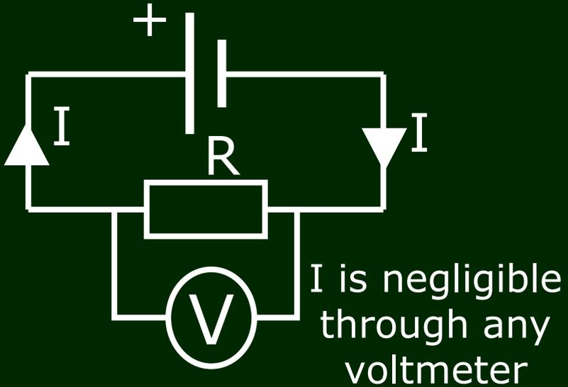
Voltmeters are designed to have very large electrical resistances.
