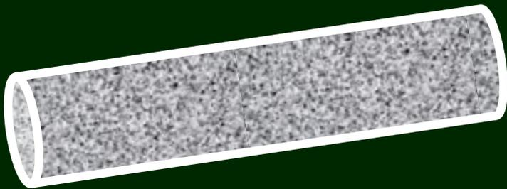
A wire has length  $L$ , cross-sectional area  $A$  and contains  $n$  charge-carriers per unit volume and each has a charge  $q$ .
