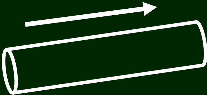
Suppose all of this charge  $Q$  flows out of this part of the wire in a time  $t$ .
