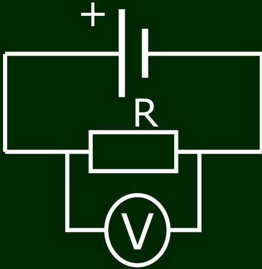
Voltmeters are always connected in parallel with other components (resistors, batteries, lamps etc).
