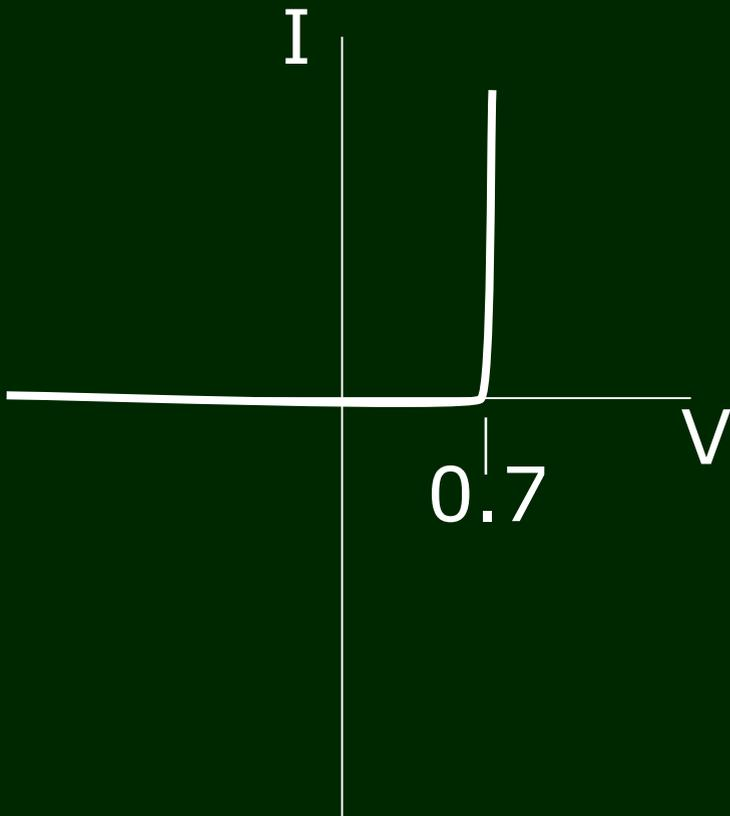
For L.E.Ds, conduction starts between 0.5 and 2V.
