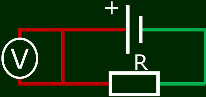
Here the voltmeter reads zero, NOT because the potential really is zero but because there is no difference between the two readings.
