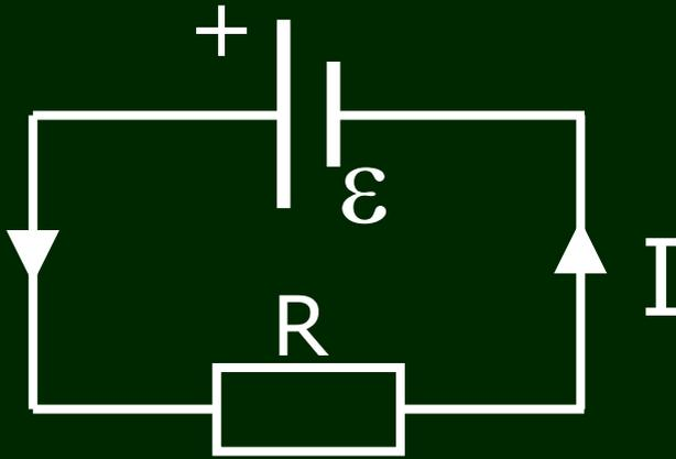
The electric current is the same at all points around a series circuit.
