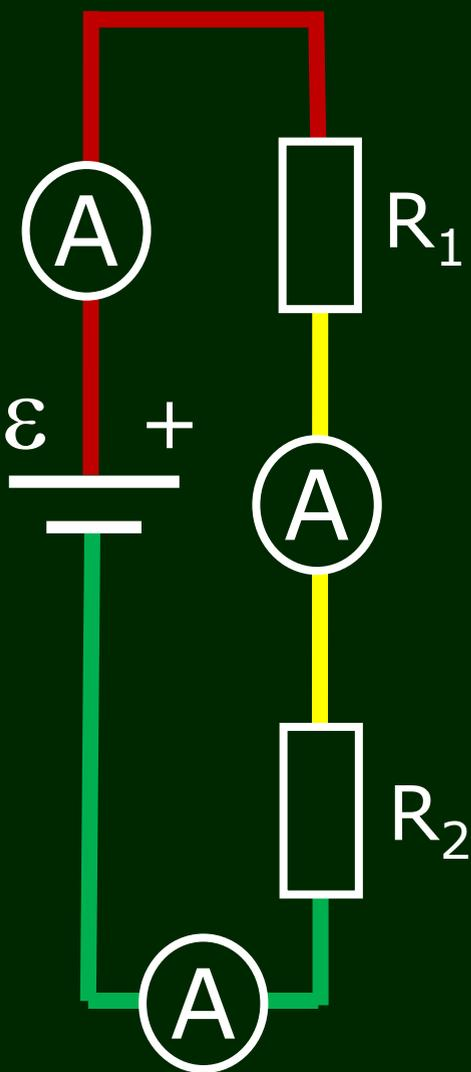
Like connecting wires, Ammeters are designed to have negligible resistances, so their presence or absence in a circuit does not affect the voltage levels (i.e. free electron spacing)
