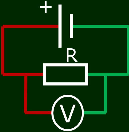
A voltmeter is a subtraction machine. It measures the potential at each terminal and displays the difference between the two readings.
