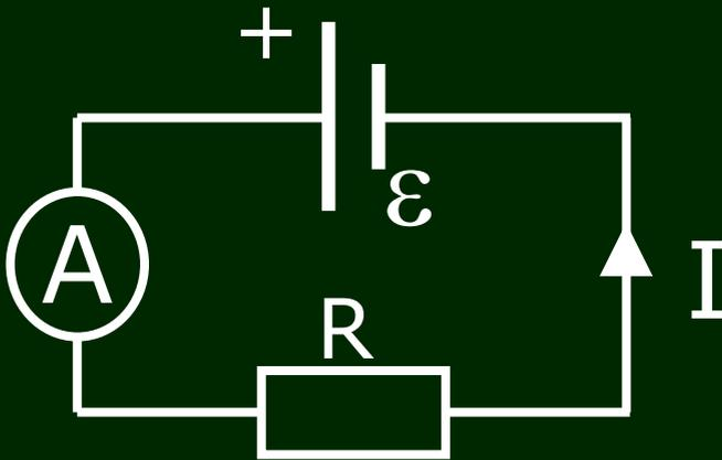
An ammeter is an electrical flow meter. It is always placed in series with other components so that current flows through it.
